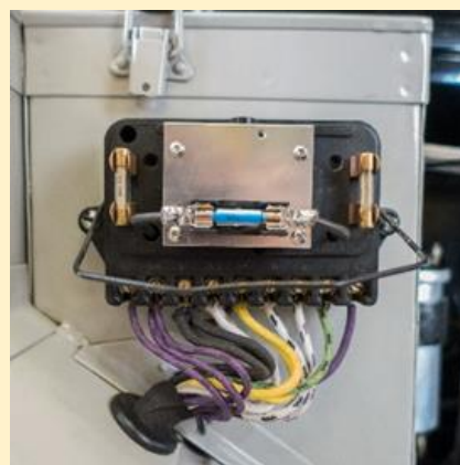
RF91 converted to solid state
